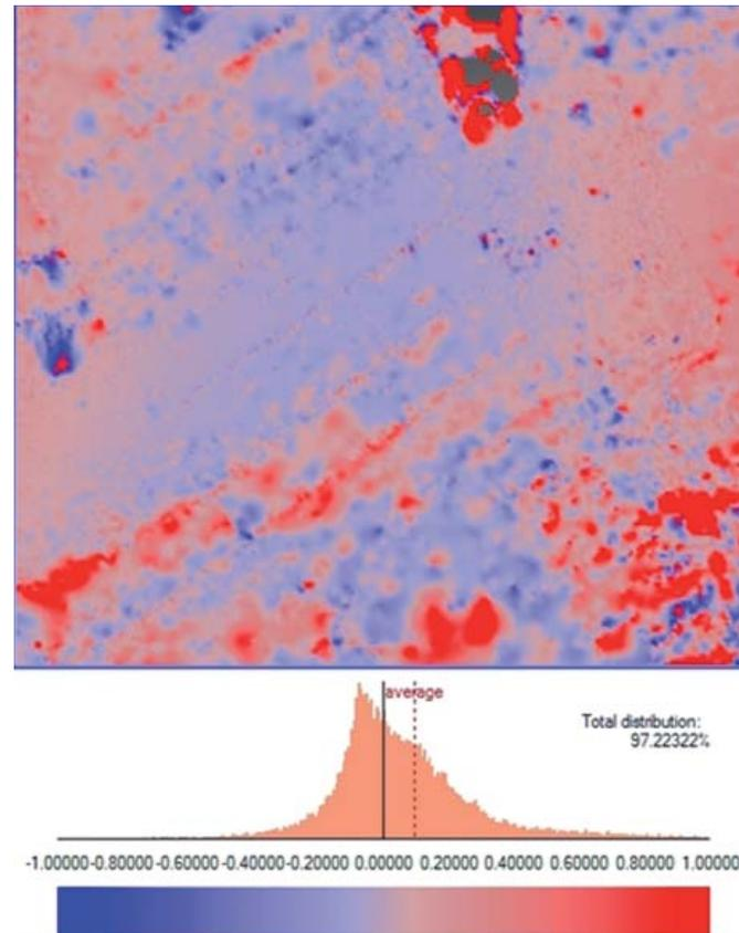
**Figure 4.** Comparison, in signed colour mode, between grid DEMs from Ideal and Ebner projects with 12 GCPs
